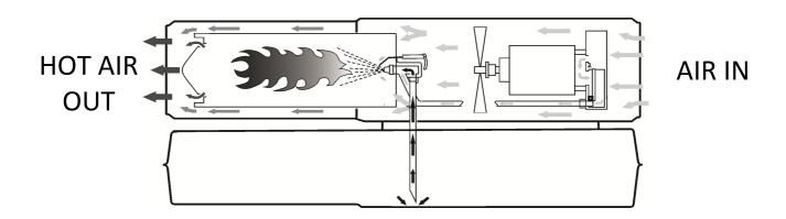
Direct oil heaters are highly efficient devices that provide large volumes of instant heat where it is required. They are best for open or well ventilated areas like factories, warehouses or construction sites. Master direct heaters are known as very efficient and robust as well as safe and easy in use.
