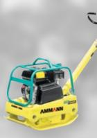
APR 2220 PETROL WEIGHT: 100 kg MAX. VIBRATING FREQUENCY: 98 Hz MAX. CENTRIFUGAL FORCE: 22 kN
