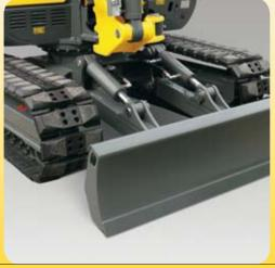
**Durable hybrid tracks** which can be driven easily over asphalt and sharp edged surfaces and whose links can be individually replaced.
