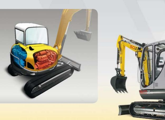
The unique construction principle of the Wacker Neuson Zero Tail machines.
